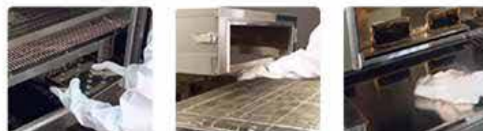
Remove the finger nozzles Pull the conveyor forward Reach and clean deep inside the oven
